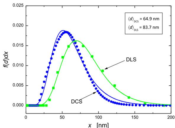
Fig. 2. Volume weighted hydrodynamic size distributions of nanoparticles measured by DLS and DCS. Solid lines were obtained by fitting the lognormal distributions to the experimental data.
