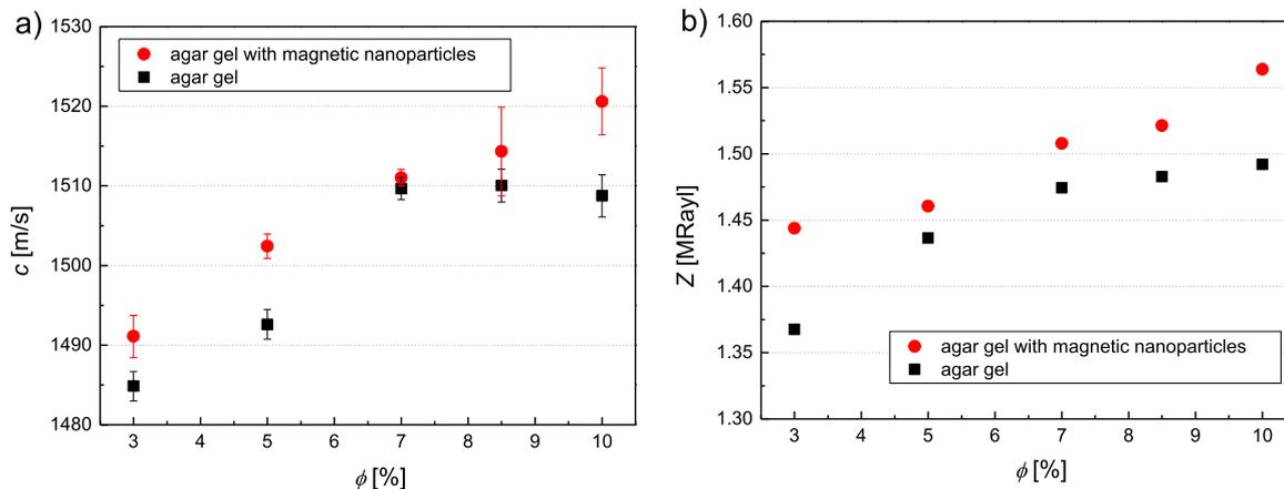
Fig. 5. Longitudinal ultrasonic wave velocity (a) and acoustic impedance (b) for different concentrations of pure agar-gel samples (squares) and agar-gel samples with magnetic nanoparticles (circles).
