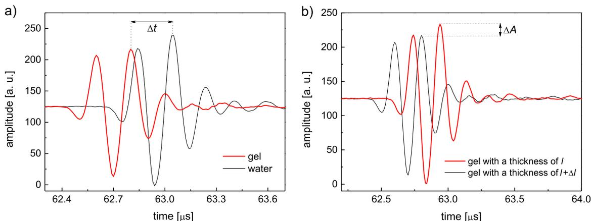
Fig. 4. Time-domain detected signals: (a) ultrasonic pulses with and without the agar samples; (b) measured pulses for two samples with different thicknesses.
