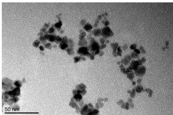
Fig. 1. TEM micrograph of synthesised Fe<sub>3</sub>O<sub>4</sub> nanoparticles.
