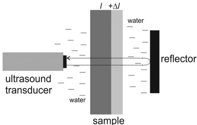
Fig. 3. Experimental setup for the velocity and attenuation of the ultrasonic wave measurements.
