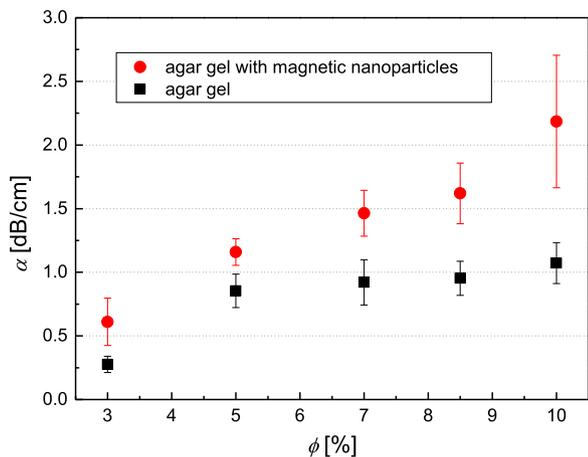
Fig. 6. Ultrasonic wave attenuation for different concentrations of pure agar-gel samples (squares) and agar-gel samples with magnetic nanoparticles (circles).
