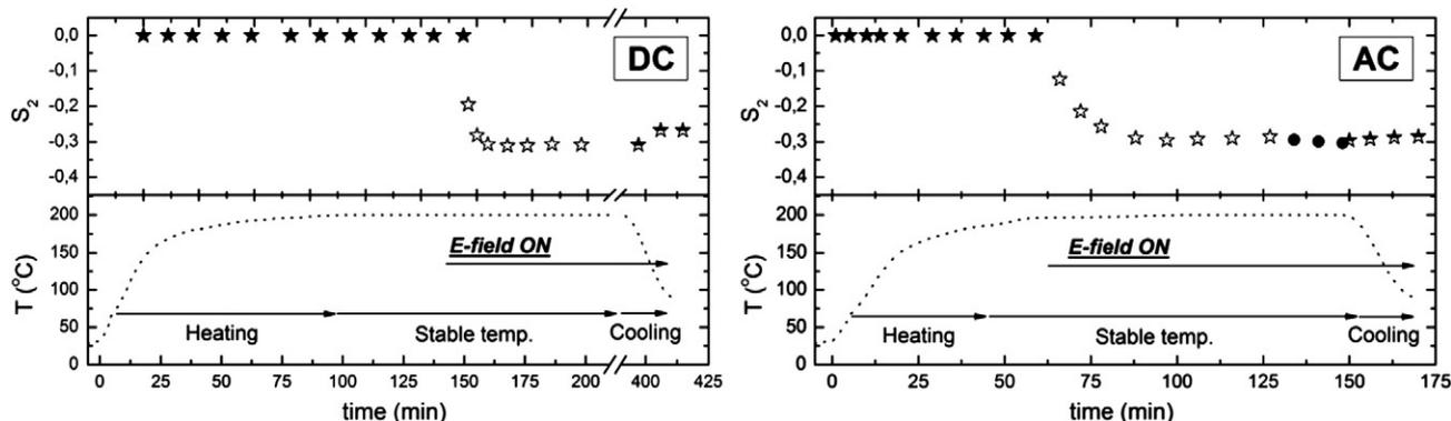
Fig. 7. Development of the degree of anisotropy as a function of time and the phase of the polymer matrix (melted vs. crystallized). A DC electric field was applied to Sample 1 (left) and an AC electric field was applied to Sample 2 (right).
