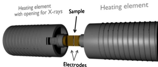
Fig. 1. Experimental set-up for SAXS measurements. Sample is placed between two copper electrodes. Two heating units are used to ensure the smallest temperature gradient between sample and environment.
