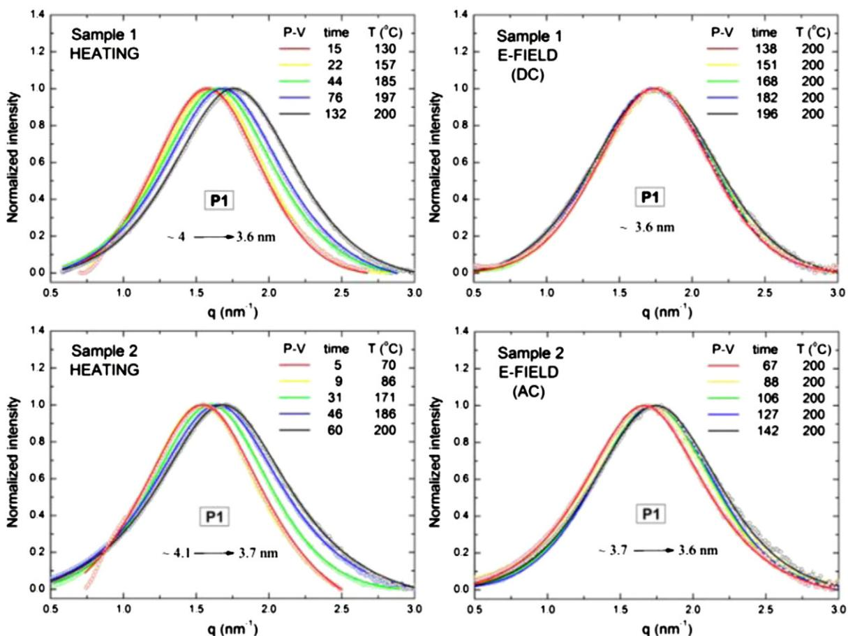
**Fig. 3.** Azimuthally integrated 2-D SAXS patterns of sample 1 (top) and sample 2 (bottom) during melting and temperature stabilizing (left); and E-field application (right). The data was fitted to Pseudo-Voigt profiles (solid lines).
