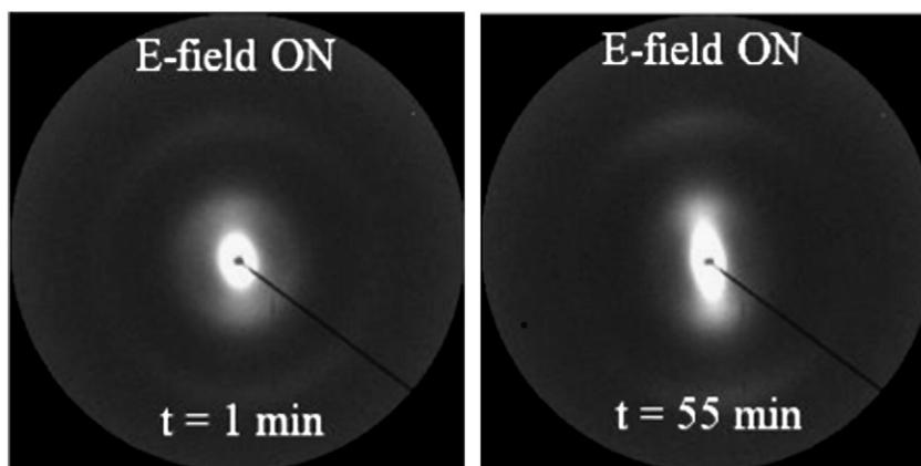
**Fig. 5.** 2-D SAXS images of a clay PP nanocomposite in melted state (around 200°C) under DC electric field of 1 kVmm<sup>-1</sup>. Very strong anisotropy can be seen (right) after 55 min of *E*-field application. The direction of the DC *E*-field is horizontal.
