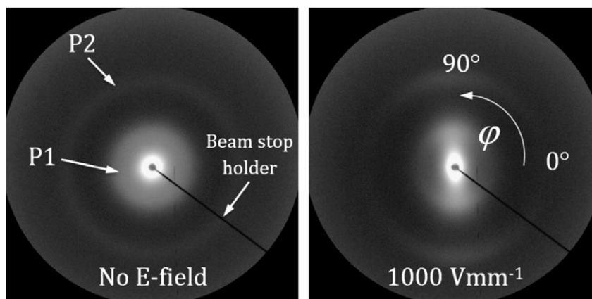
**Fig. 2.** 2-D SAXS images of a PP-organoclay nanocomposite in melted state (around 200°C) before (left) and after (right) application of an AC electric field of 1 kVmm<sup>-1</sup>, 100 Hz for 5 min. Strong anisotropy can be seen in the right image. The direction of the AC E-field is horizontal.
