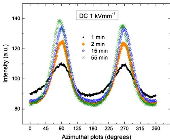
**Fig. 6.** Azimuthal plots of the first Bragg peak amplitude ( $q_1$ , polymer intercalation) for PP-clay sample under DC electric field of 1 kVmm<sup>-1</sup>. The degree of anisotropy grows starting immediately after the application of the electric field.
