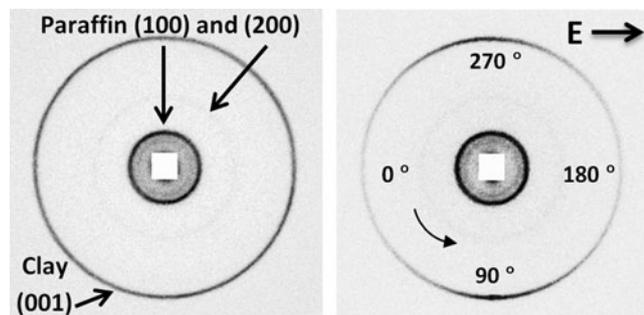
FIG. 1. 2D WAXS patterns from paraffin–clay composites without (left) and with (right) an applied external electric field of  $250 \text{ V/mm}$ . The outermost ring from clay becomes anisotropic indicating that clay particles are aligned with their stacking direction perpendicular to the electric field lines.
