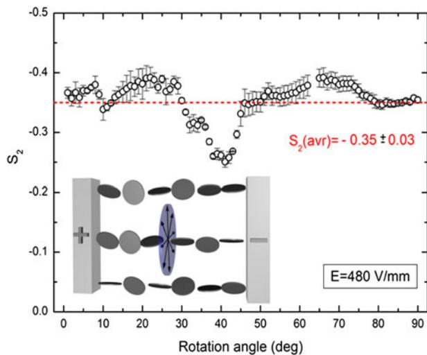
FIG. 2. The nematic order parameter calculated for different rotation angles. The average  $S_2$  value is indicated as a dashed line. The inset shows a sketch of the clay alignment in a so-called antinematic configuration (see text for details).
