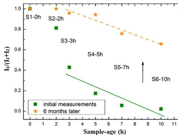
FIG. 6. The ratios  $I_1/(I_1 + I_2)$  between magnitudes of 0 WL and 1 WL peak intensities for six samples (Sample Batch 2). Their values are in the range of 0–1, where 0 indicates the pure dehydrated state, 0.5 is obtained when the number of clay particles in the two states are equal, and 1 depicts the pure monohydrated state.
