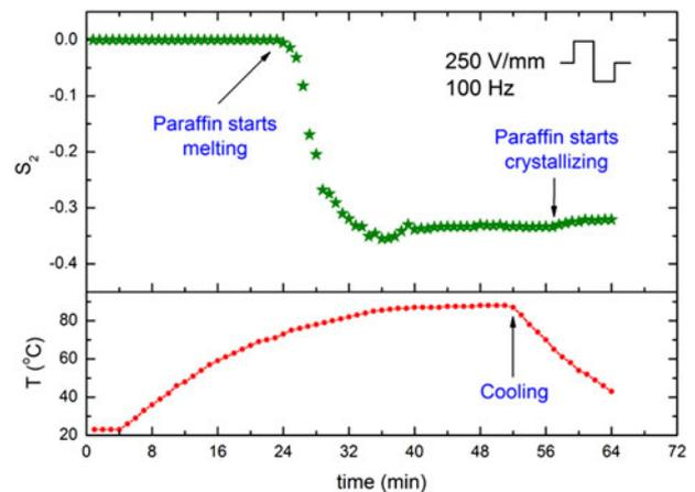
FIG. 4. Development of the anisotropy in the system expressed by changes in the nematic order parameter  $S_2$ .
